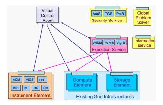
Figure 1: The Components of the GRIDCC architecture
