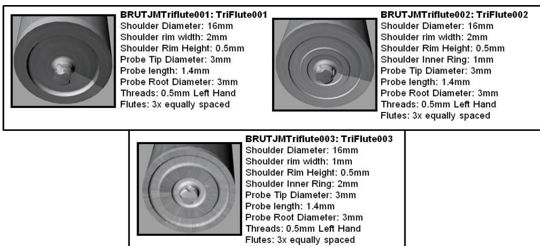
Figure B1.3, Triflute Tool Specifications.
