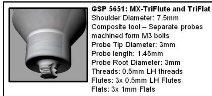
Figure B1.4, GSP 5651 tool specifications.
