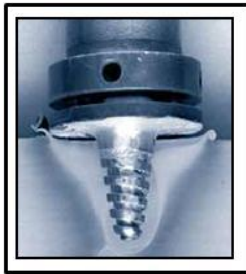
Figure A1.7, TWI Designed Whorl™ FSW Tool [1, 111].
