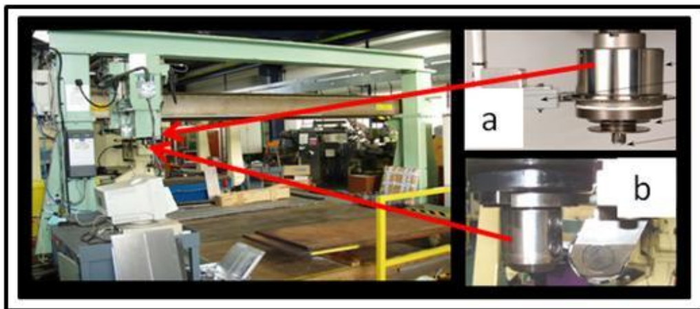
Figure 6.2, FW22 FSW Machine Inset: a) LoStir Force Monitoring System, b) Conventional Tool Holder and Tool Heel Roller.
