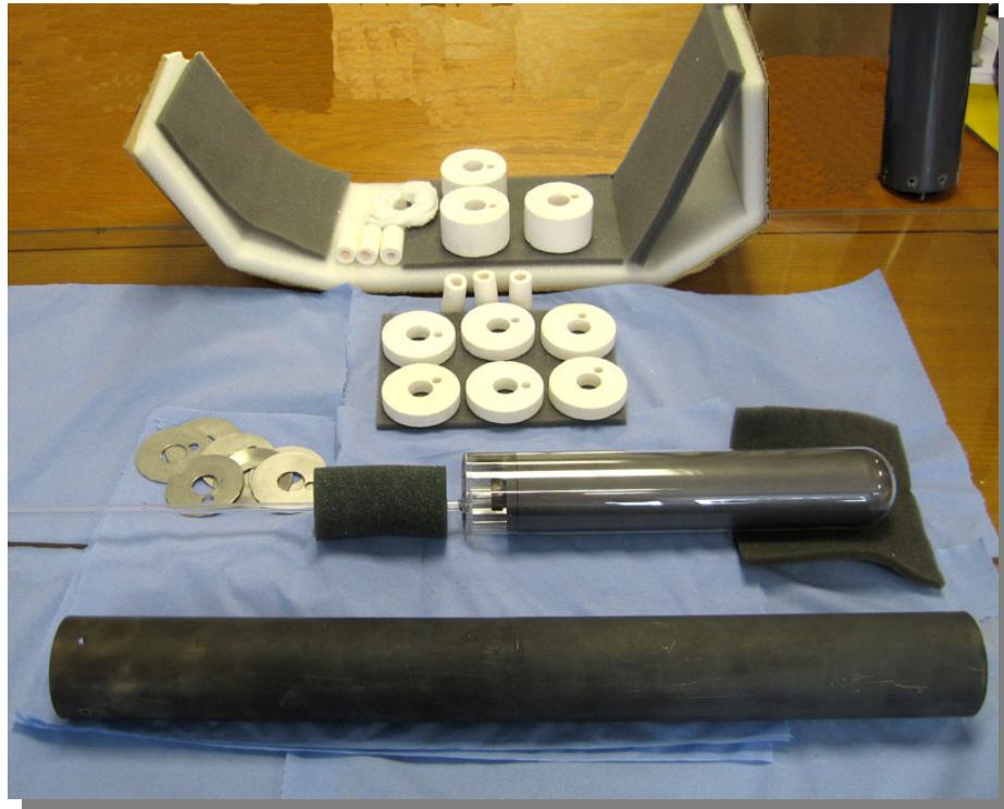
Figure 5.3 Components of the original Spanish tin opened-“sealed cell” assembly.
