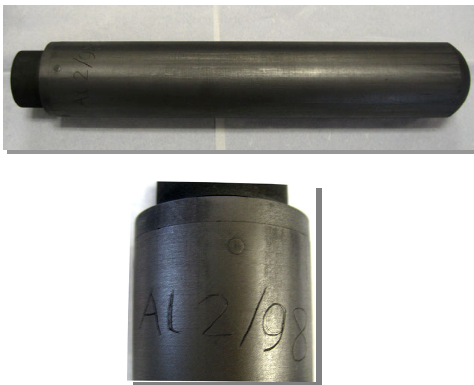
Figure 5.16 Aluminium 298 fixed-point ingot.
