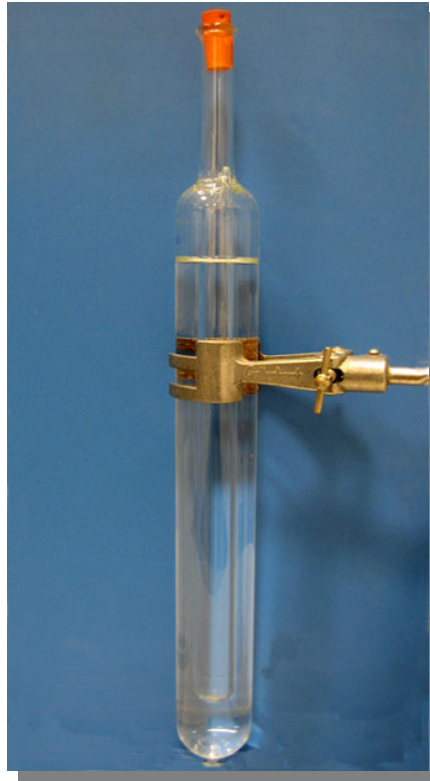
Figure 5.1 NPL small water triple point cell.
