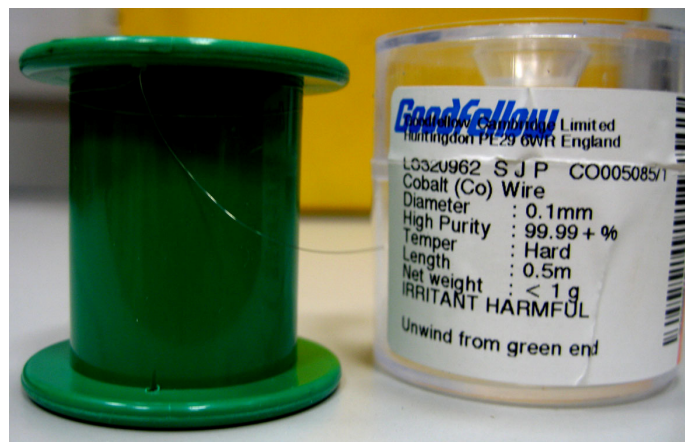
Figure 5.7 An example of the metal wire used as an impurity for doping in Spanish tin cell.
