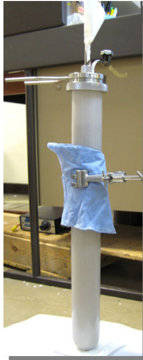
Figure 5.18 “undoped” Al 298 fixed-point opened cell.
