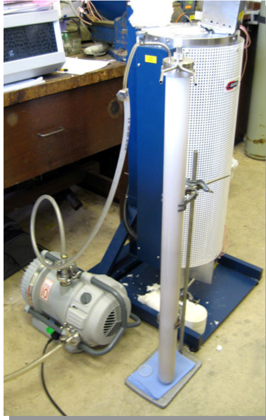
Figure 5.8 System for baking the bricks and graphite discs at 1100 °C.
