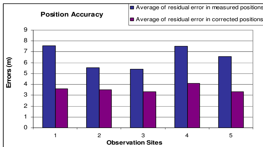
Figure 3.3: GPS Position accuracy achieved using standard GPS and DGPS (AL Nabhan et al., 2008)
