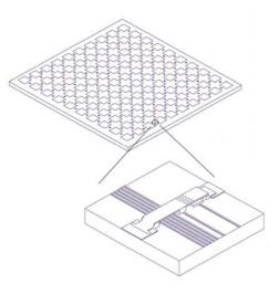
Fig.1. Microstrip array antenna and the expanded view of the ohmic RF MEMS Switch.
