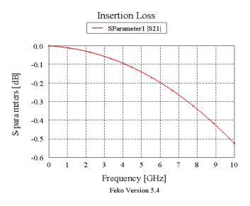
Fig.8. Insertion loss of the proposed switch in the ON state.
