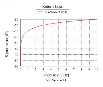
Fig.7. Return loss of the proposed switch in the ON state.
