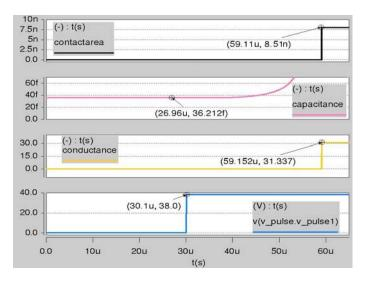
Fig.5. Contact area (nm), capacitance (fF) and conductance (S) of the proposed switch.
