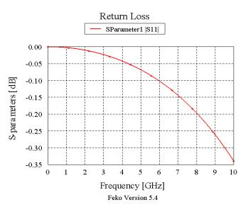
Fig.9. Return loss of the proposed switch in the OFF.
