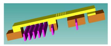
Fig.2. The proposed ohmic RF MEMS Switch.
