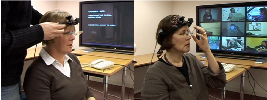
Figure 7.4: User testing in progress using eye-tracking hardware
