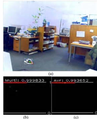
Fig. 7. (a) A radio controlled model car has almost parallel vectors. b) While the car is moving forwards and backwards, the averaged \cos\theta from each frame is fairly close to 1. c) The average of every frame's \cos\theta value is also considerably close to 1.
