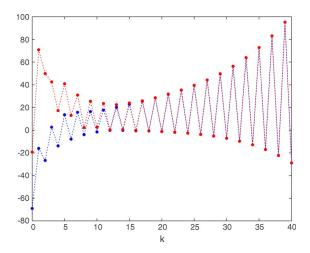
Fig. 3. State trajectories of  $x_{11}$  and  $\hat{x}_{11}$ .
