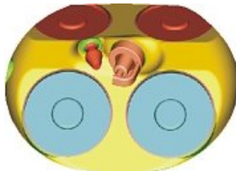
Figure 3.1 Combustion Chamber of Prototype Orbital Cylinder Head (Orbital Engine Corporation Ltd)
