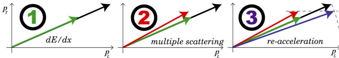
Figure 1.3: Ionisation cooling 52 . The overall momentum of the beam is reduced by an absorber material before the longitudinal momentum of the beam is restored by a RF cavity, reducing the overall emittance of the beam.
