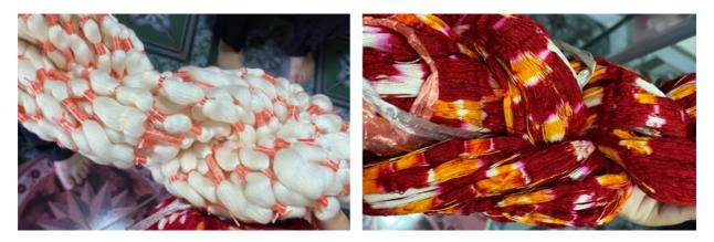
Figure 5.29 Outsourced pre-tie-died yarns (left) and after dyeing (right)
