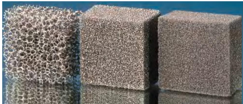
Figure 2.51. Titanium implants with differing porosities (Edosa et al., 2022).
