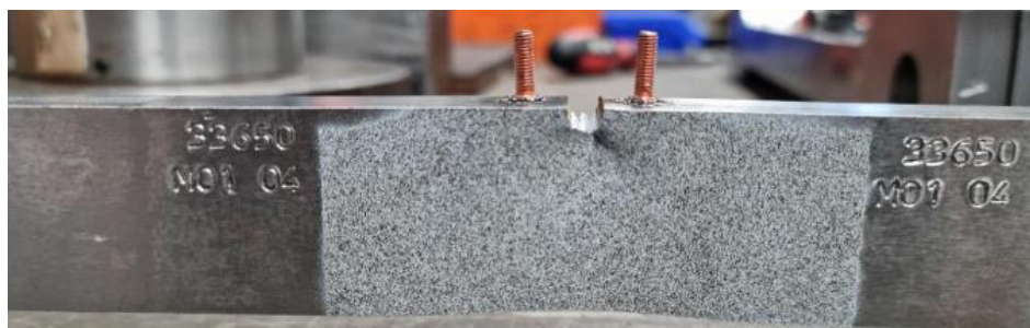
Figure 3.14: Pin-loaded SENT specimen, a/W = 0.1 tested to maximum load
