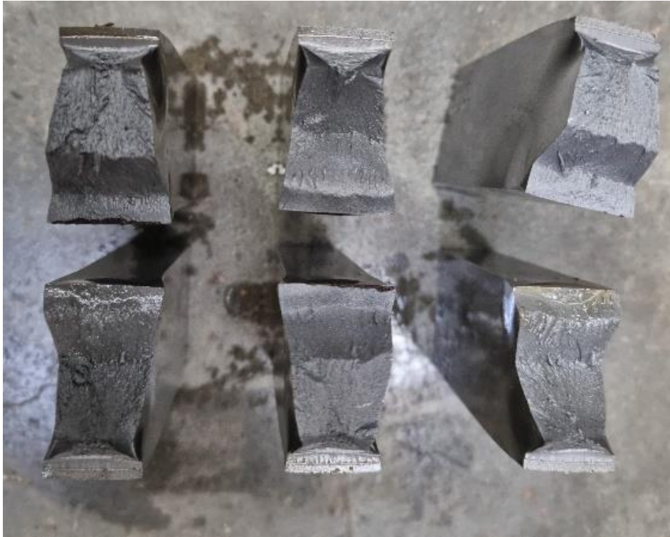
Figure 3.21: Fracture surface of SENB with crack depth, a/W = 0.1 tested at -120^{\circ}\text{C}
