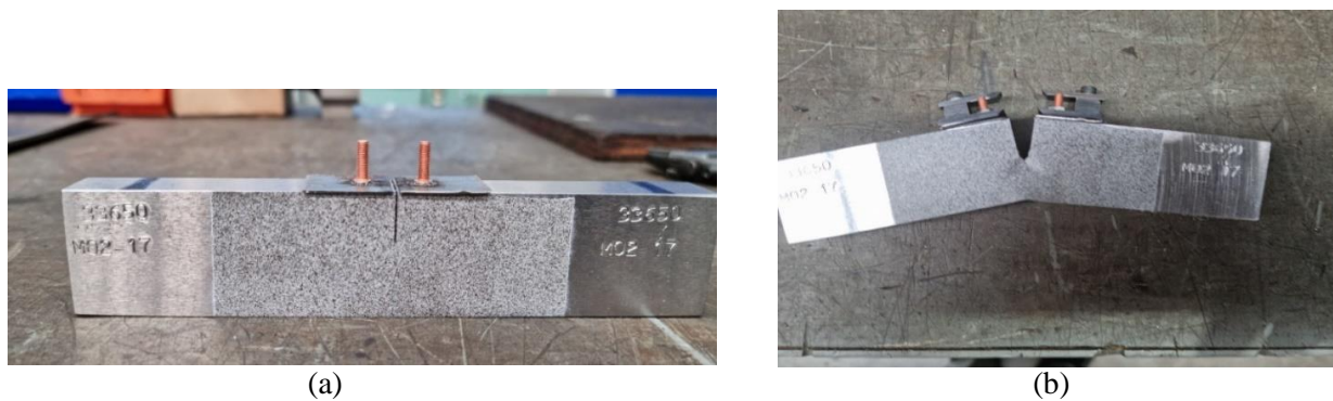
Figure 3.16: SENB specimen for room temperature test, a/W=0.5 : (a) Speckle pattern generated on the surface of for DIC measurement (b) tested to maximum load
