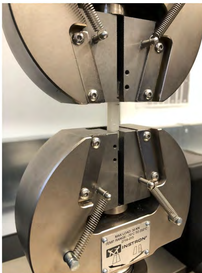
Fig. 24 The setup of tensile properties testing on the Instron machine
