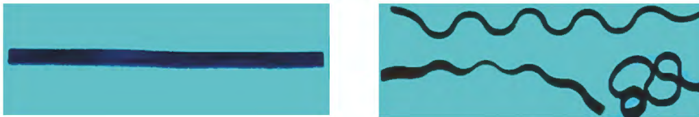
Figure 2-32. An example of bending, twisting, and wrinkling (Ge et al., 2013).
