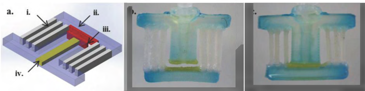
Figure 2-6. A smart valve created using 4DP (Bakarich et al., 2015).
