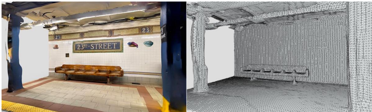
Figure 4.4 LiDAR Textured Mesh (left) and Wireframe (right)
