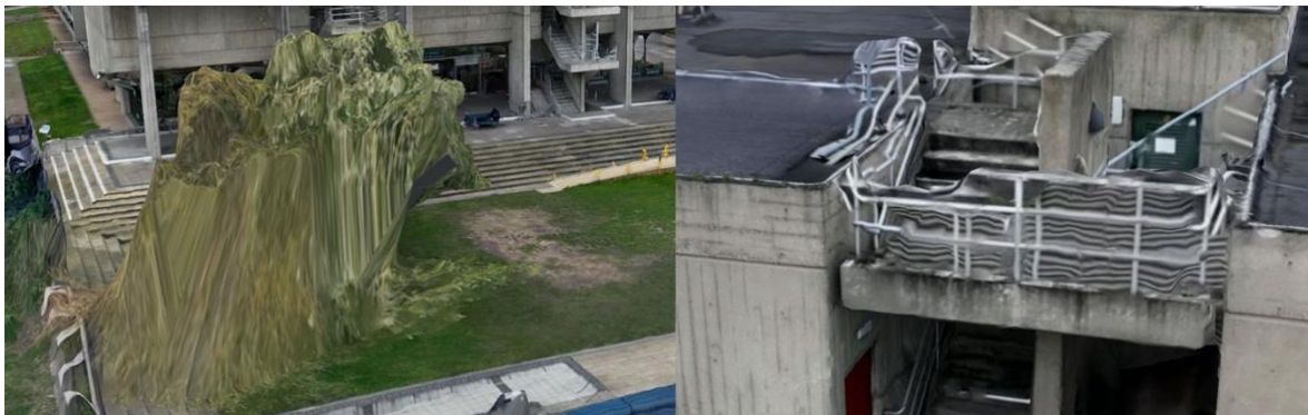
Figure 7.29 Capture Artefacts: Tree Branches and Leaves (left), Handrails (right)
