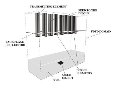
Fig. 1. FDTD Model of a PRSF-SPR system
