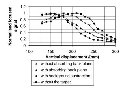
Fig. 2. Vertical focusing through target location
