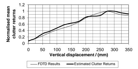
Fig. 3. Comparison of FDTD clutter echoes with the estimated clutter
