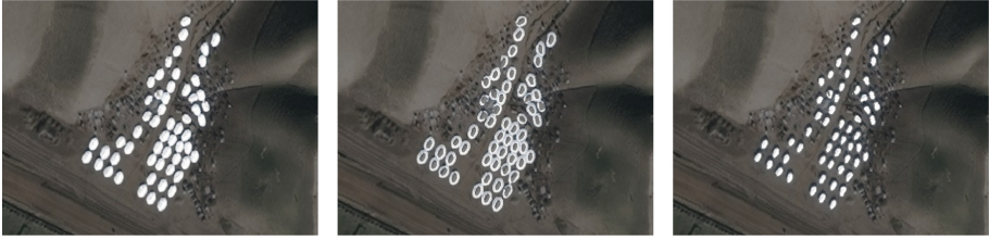
Fig. 6. Left: Segmentation mask produced for NRC tents in a camp near Qala'e'Naw. Centre: Edges mask produced for the same image. Right: The final output mask.
