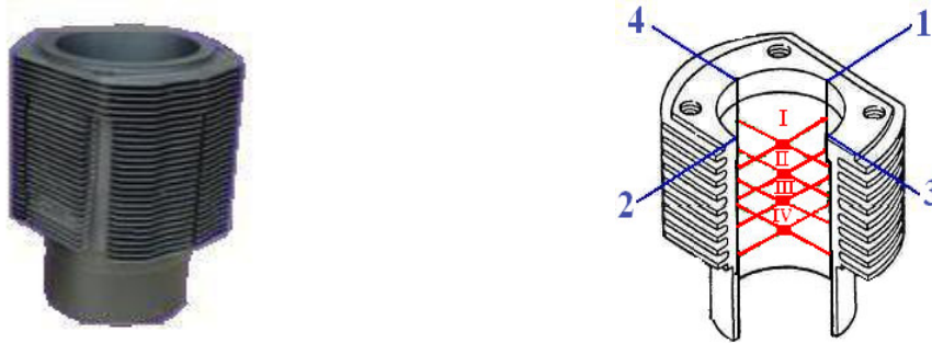
Fig. 2. (a) Cylinder configuration (b) Locations for roundness and straightness measurements Fig. 2. Engine cylinder configuration and locations of measurements
