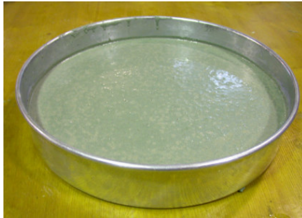
Fig. 6. Mixture of SiC abrasive and SSB in a mould
