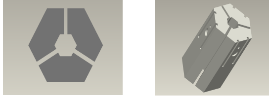
Fig.3. Top and general views of the module's hexagonal body.
