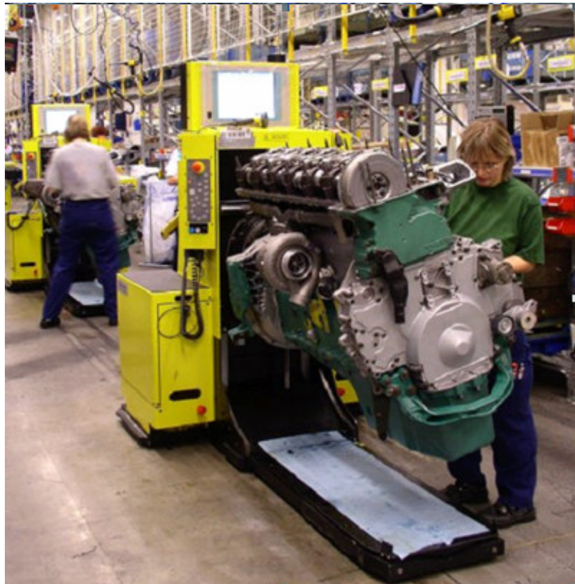
Fig. 1. The AGV/carrier and its cargo, a diesel engine.
