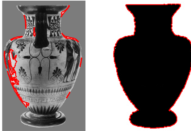
Figure 3.2: Binarization benefits. L: a grey-scaled image, with contours (red) obtained via a Marching Squares algorithm. R: A binarized image, with contours extracted, once again, using Marching Squares. Here, the contour extraction computation on the binarized image was approximately 5.5 times faster than the implementation on the grey-scale image.
