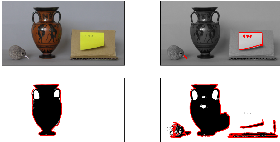
Figure 3.3: Top left: a photograph of an ancient Greek vase (alongside a kiwi toy for scale and some card to label the picture), taken by Stephen Marsland, in the Classics Museum 66 at Victoria University of Wellington. Bottom left: a binarized version of the original photograph, and an outline contour of the vase, overlaid in red. Our own binarization algorithm, which also incorporates the essence of segmentation, is used in this particular example, which we will outline in the subsequent sections. Top right: a grey-scale version of the original photograph, and the top contours obtained after contour extraction on the grey-scale image. Bottom right: contour extracted and plotted on top a binarized version of the original photograph, using a popular binarization algorithm, Otsu’s thresholding method, ( Otsu, 1979 ). Although our binarization algorithm has done rather well in binarizing the original image, the contour extraction algorithm was still susceptible to some noise caused by a shadow, which can be seen on the lower-right side of the vase. And the same can be said for Otsu’s thresholding method, where the resulting vase contour is more affected by the shadow. However, the success of both binarization algorithms, particularly our one, can certainly be praised, when the resulting contours are compared to the contours in the top right plot, where a method of image binarization was not employed prior to contour extraction. The basis of the contour extraction steps on all images was the Marching Squares algorithm, ( Lorenson and Cline, 1987 ), which we will describe in more detail, later on in this chapter.
