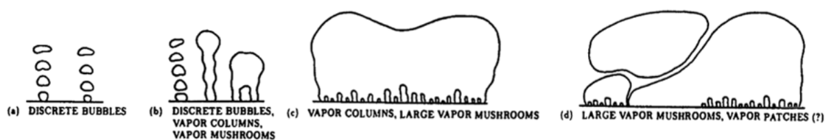
Figure 4-12. Bubble phenomena during nucleate boiling regime, from Gaertner [95]
