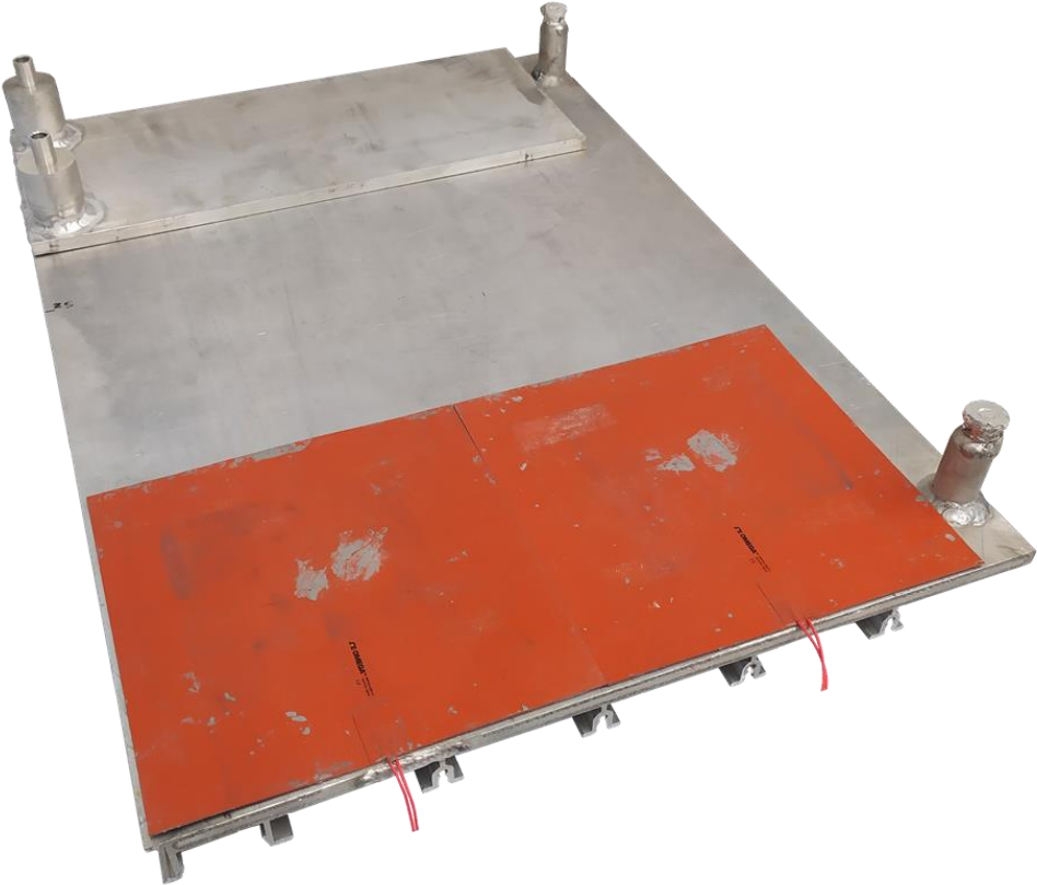
Figure 3-15. Multi-channel flat heat pipe assembly with silicon flat heaters as a heat source and a cooling manifold as a heat sink
