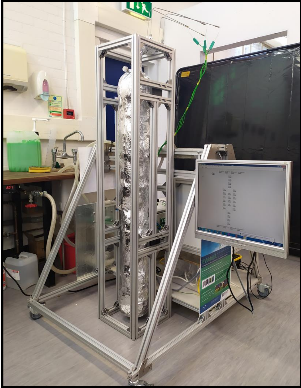
Figure 3-22. Experimental test bench while testing the three-leg multi-channel heat pipe
