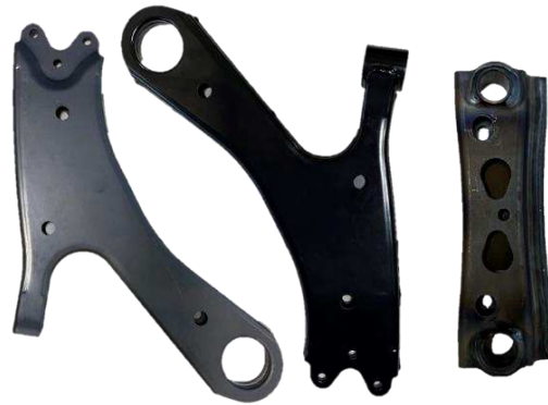
Figure 5 The proposed metallic chassis components by Gestamp that will be strengthened with thermoplastic composite patches using PCM joining method.
