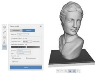
Figure 11. Photogrammetry using Autodesk Recap Photo
