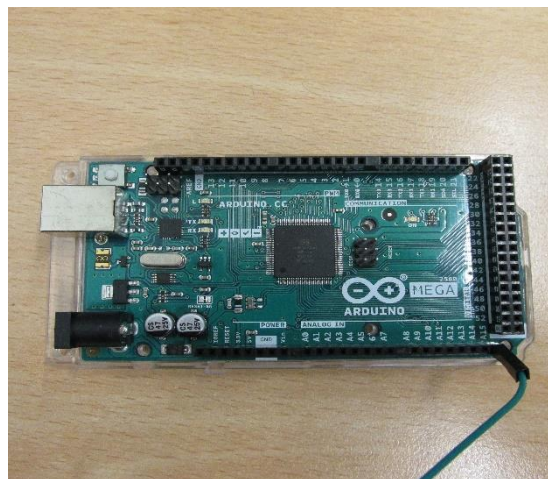
Fig. 73 Arduino Mega 2560 Control Board (Fox.A,2019)
