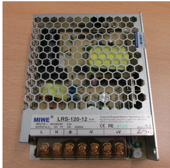
Fig. 74 240v/12v 10A power supply (Fox.A,2019)
