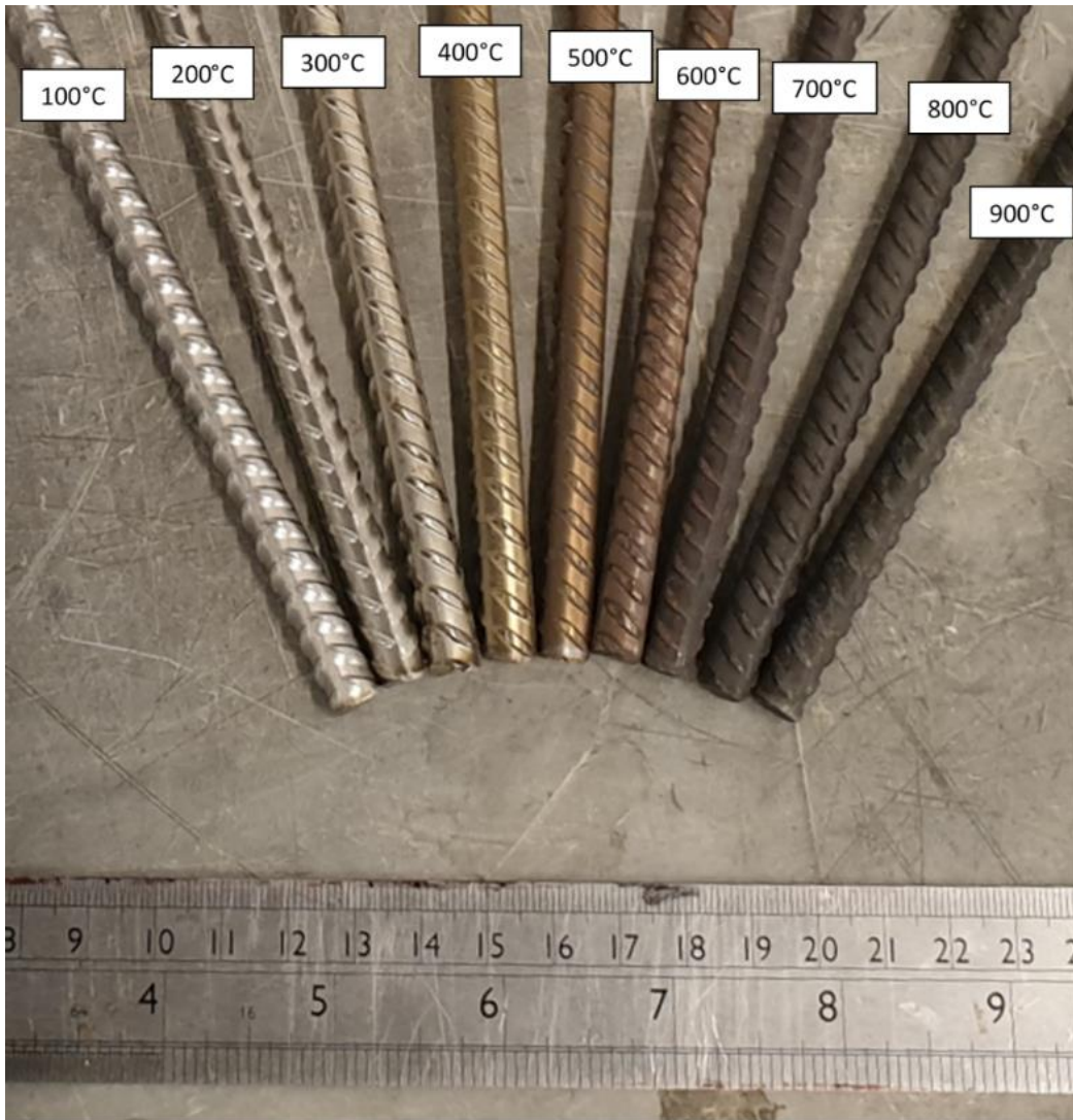
Figure 3-1: Grade 1.4301 following exposure to elevated temperature and subsequent cooling.
