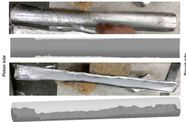
145 Fig. 7 Comparison of solid shape in sleeve between filling tests and model calculations
