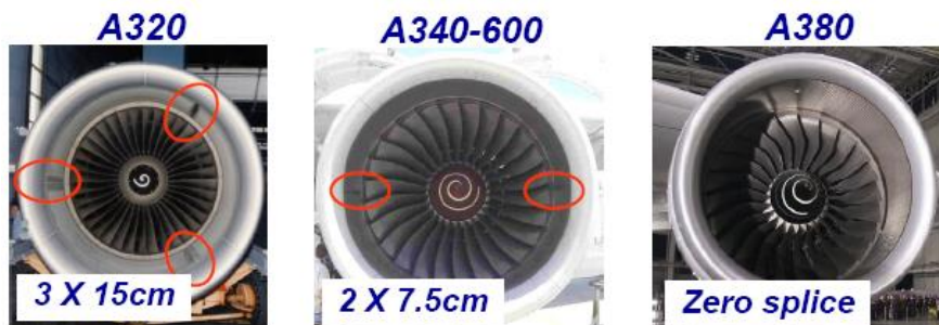
Figure 1.2 - Examples of engine intake technology improvement. Photo courtesy of Rolls Royce (7).
