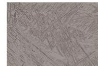
Figure C.1 Microstructure images of Ti6Al4V/AA6061 HS-LR joints at the crown area with varied magnifications.
