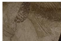
Figure C.1 Microstructure images of Ti6Al4V/AA6061 HS-LR joints at the crown area with varied magnifications.
