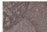
Figure C.1 Microstructure images of Ti6Al4V/AA6061 HS-LR joints at the crown area with varied magnifications.
