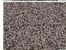
Figure C.1 Microstructure images of Ti6Al4V/AA6061 HS-LR joints at the crown area with varied magnifications.
