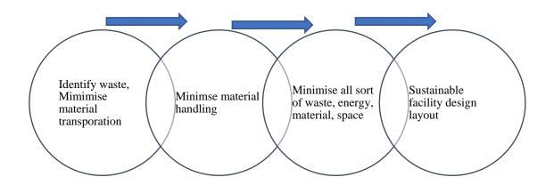
Figure 2.13 The procedure of SFLD
