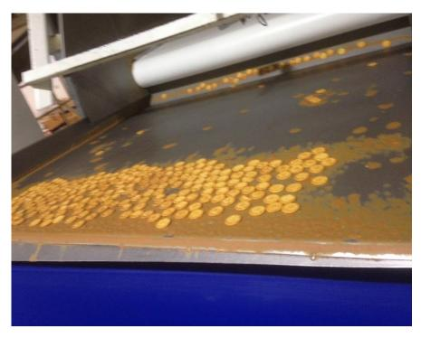
Figure 6.24 Lower portion of storage conveyor with flavour particles
