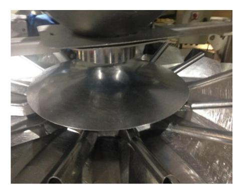
Figure 6.13 Top cover above lower feeders
