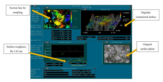
Figure 6.48 Surface roughness is 1.65 um of the existing Metal sample used in the company
