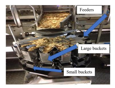
Figure 5.6 Production machine with its parts
