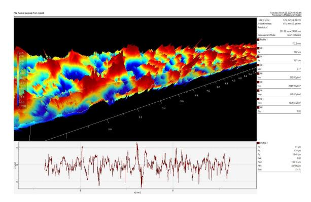
Figure 4.27 Sample surface texture with oil coating
