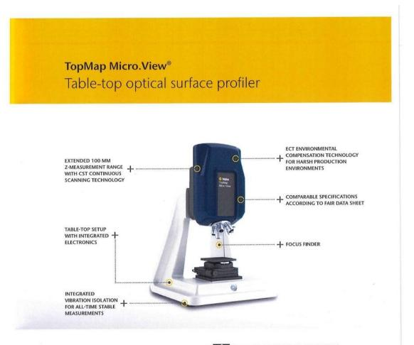
TopMap Micro.View<sup>®</sup> is an easy to use and compact optical profiler. Combine exceptional performance and affordability with this powerful metrology solution. An extended 100 mm Z-measurement range with CST Continuous Scanning Technology allows complex topographies to be measured at nm resolution.This conventient table-top setup features integrated electronics, with the smart focus finder simplifying and speeding up the measurement procedure.
