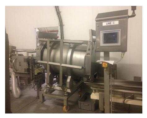
Figure 6.33 Flavour mixer drum on the production line
