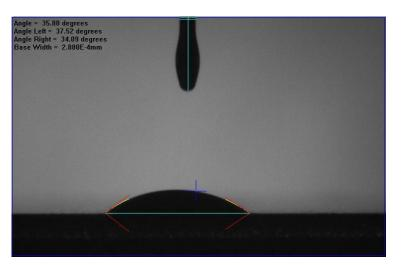
Figure 4.31 Contact angles with cooking oil
