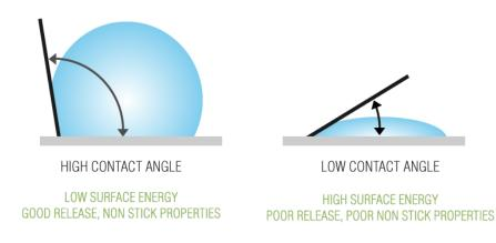
Figure 5.14 Proposed contact angle on proposed surface with low surface energy [100]
