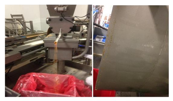
Figure 6.36(a) Flavour mixer drain to bin bag. (b) outside side of flavour mixer with flavour depoist on the surface
