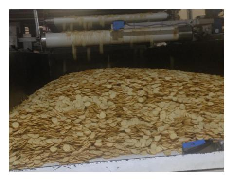
Figure 4.14 Storage vibrating metal conveyor while in operation
