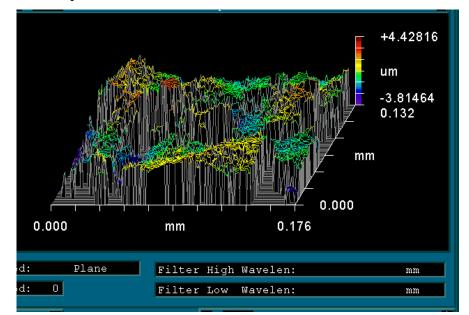
Figure 3.6 3D surface waviness diagram
