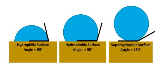
Figure 5.12 Water repellent surface with different angles
