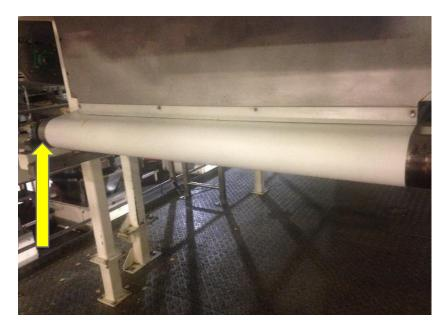
Figure 4.16 Proposed location where fixed cleaning brush can be Mounted to clean soft fabric conveyor during operation
