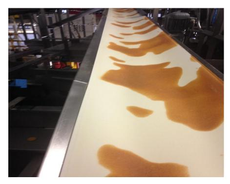
Figure 6.28 Soft conveyor belt transporting crisps from oven to storage conveyor
