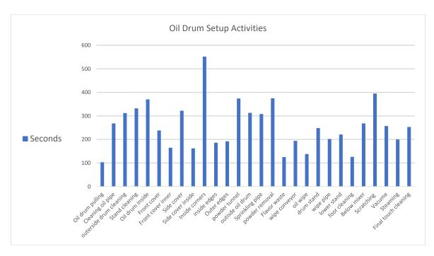
Figure 4.4 Activities in oil mixer drum setup and cleaning
