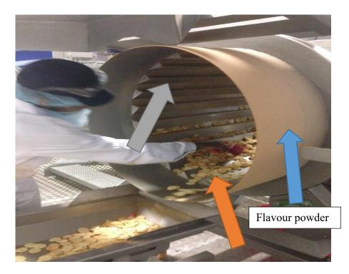
Figure 4.17 Flavour mixer drum manual cleaning process from inside
