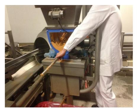
Figure 6.37 Disassembling of flavour tank
