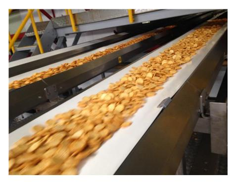
Figure 6.2 Soft conveyor belt transporting crisps from oven
