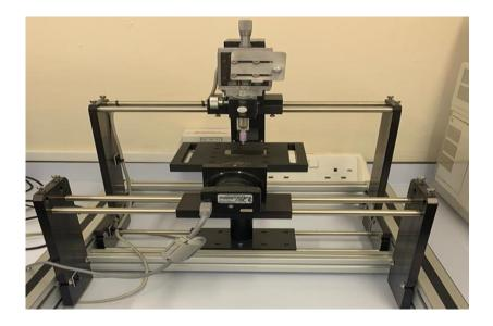
Figure 4.29 Instrument for contact angle measurements
