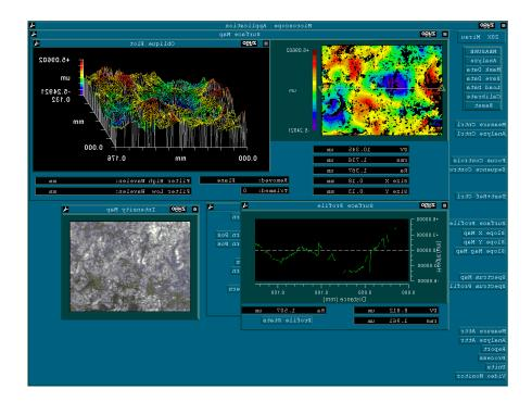
Figure 3.7 3D surface parameters and dimensions
