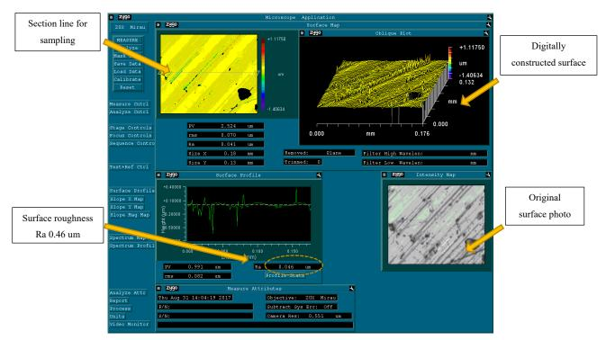
Figure 6.49 Smooth surface roughness 0.046um
