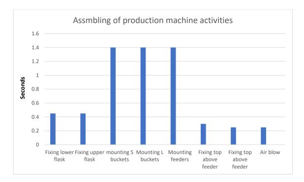
Figure 6.22 Assembling of production machine activities
