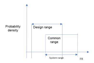
Figure 2.7 FRs design range diagram
