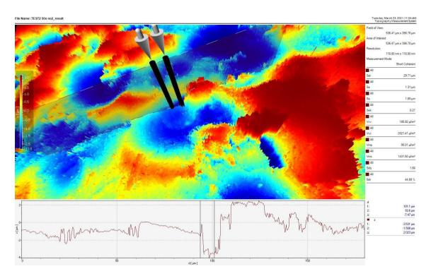
Figure 5.10 Surface roughness parameters of the sample surface
