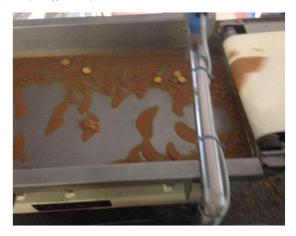
Figure 6.39 Metal vibrating conveyors before cleaning
