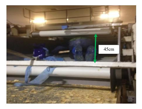
Figure 1.5 Photograph highlighting limited access during cleaning
