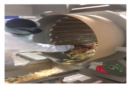
Figure 6.35 Manual removal of crisps from flavour mixer
