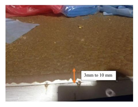
Figure 1.4 Thick material sticks on the storage conveyor surface
