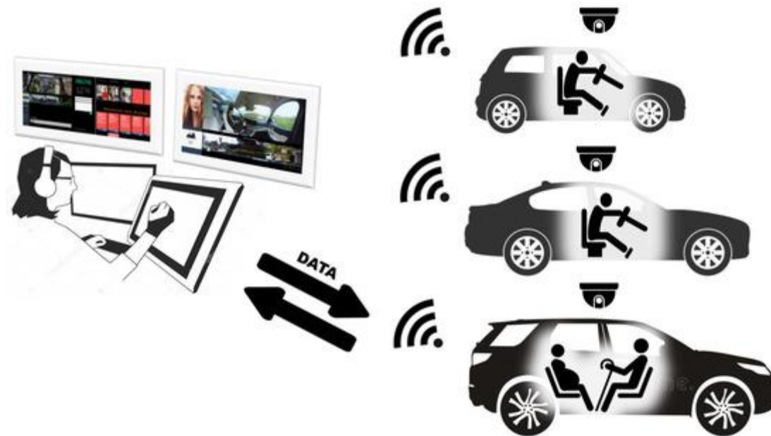
Figure 28: Remote automotive UX systems support in UX research and design by observing; interacting with synchronous or asynchronous data concerning the context of the car; and communicating in real-time with the passengers or the drivers.
