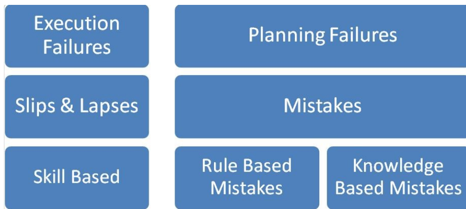
Figure 2.1: Reason's Reason (1990) Slips, Lapses, Mistakes mapped to Rasmussen's Rasmussen (1983) Skill-based (SB), Rule-based (RB) and Knowledge-based (KB) error types
