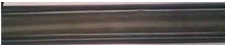
Figure 2.5 The flow pattern regimes by Singh et al. (2009), using water with a horizontal microchannels tested different heat fluxes and a mass flow rate of 2.2 ml/min,.
