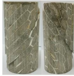
The failure patterns of laboratory physical specimen in \beta = 45^\circ , the direction parallel to column axis (Ji et al. 2017)
