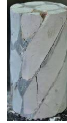
The failure patterns of laboratory physical specimen in \beta = 30^\circ , the direction parallel to column axis (Xiao et al., 2014)
