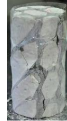
The failure patterns of laboratory physical specimen in \beta = 45^\circ , the direction parallel to column axis (Xiao et al., 2014)
