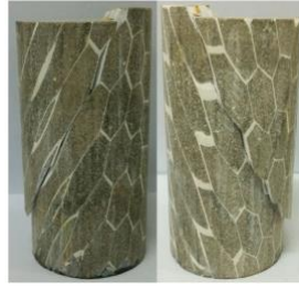
The failure patterns of laboratory physical specimen in \beta = 30^\circ , the direction parallel to column axis (Ji et al. 2017)
