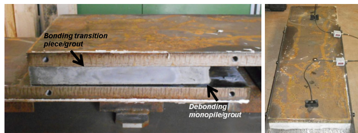
Figure 3: Propagation mock up side and AE sensors coupling.
