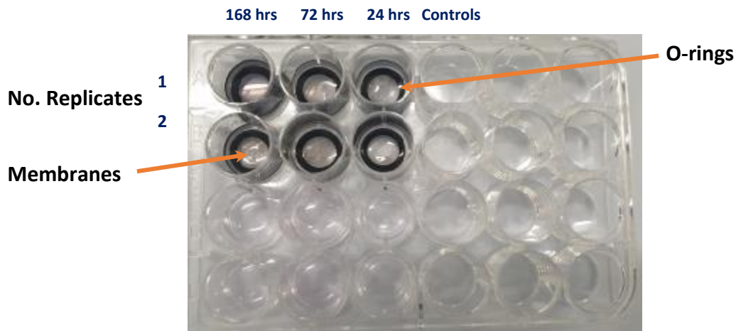
Figure 5.4 24 well plate with membranes held down in the well with nitrile O-rings to prevent samples from floating during experiments.
