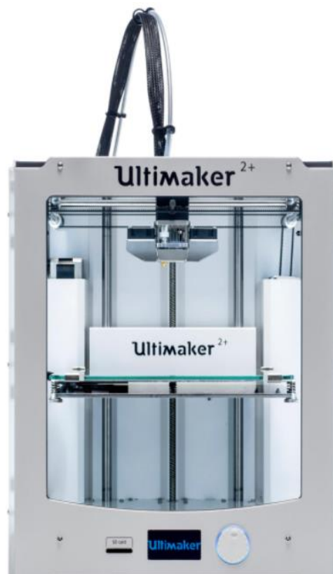
Figure 2.20 Ultimaker 2+ is an example of FDM printer, which uses filaments to build an object through material extrusion process (Professional 3D printing made accessible | Ultimaker, 2011).
