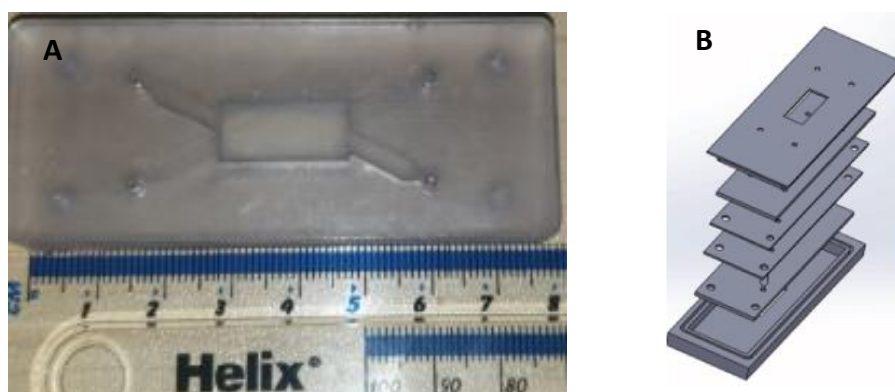
Figure 6.2(A) 3D printed VOC platform in VeroClear; (B) Design concept for TPU VOC platform.
