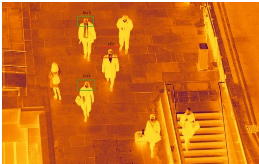
Fig. 6. Validation dataset of thermal images with temperature sensing
