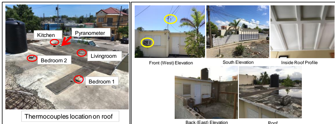
Figure 3-6: Photos of Portmore, Jamaica case study house. The position of the shielded ventilated HOBO UX100-003 data logger and the non-functioning air-conditioned unit is shown (yellow circle in the right picture) (photos provided by UTech, Jamaica).
