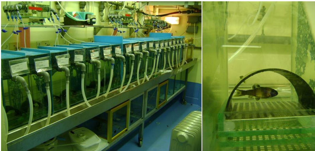
Figure A 4. Pair Breeding Test fish tank room set up with sets of 8L tanks fed dilution water/EE2/effluent via 6- or 8-hole mixing chambers. Each tank contained a spawning chamber and housed a pair of fathead minnows.
