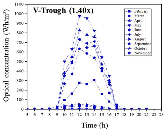
Fig. 9. The predicted optical performance of ACPC, CPC, and V-Trough concentrators.
