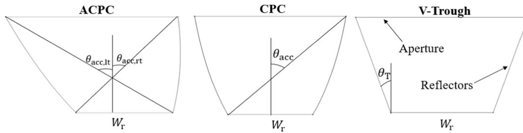
Fig. 1. Cross sectional view of the optical concentrator geometries studied.
