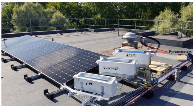
Fig. 4. The in house developed LCPV panels and conventional flat PV panels installed at the outdoor test facility within Brunel University London.
