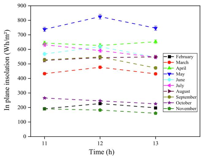
Fig. 6. The in-plane insolation incident on the aperture of LCPV panels at 11:00 AM, 12:00 PM and 1:00 PM.
