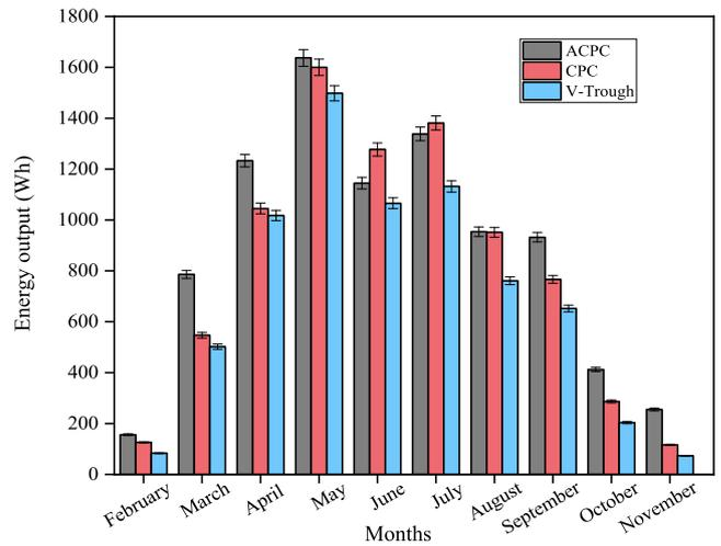
Fig. 10. The measured electrical energy output of the LCPV panels developed.
