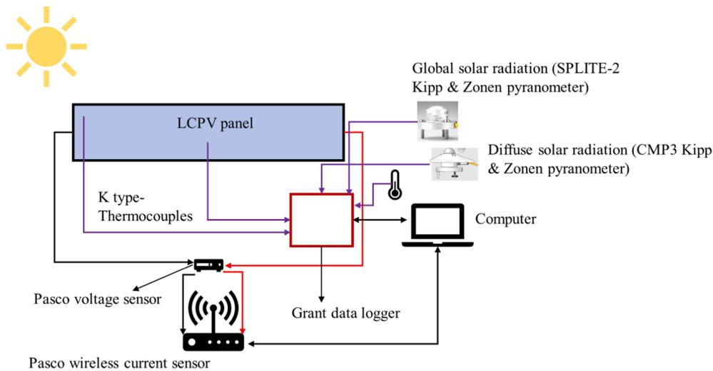
Fig. 3a. The schematic of the developed LCPV panel with the monitoring equipment.
