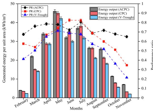
Fig. 15. Performance ratio and the generated energy output per unit cell area of the LCPVs studied.
