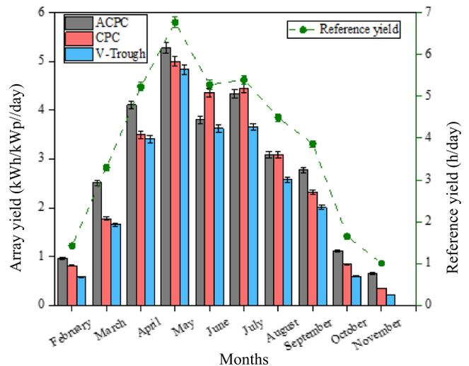
Fig. 13. The array and reference yields of the developed LCPV panels.
