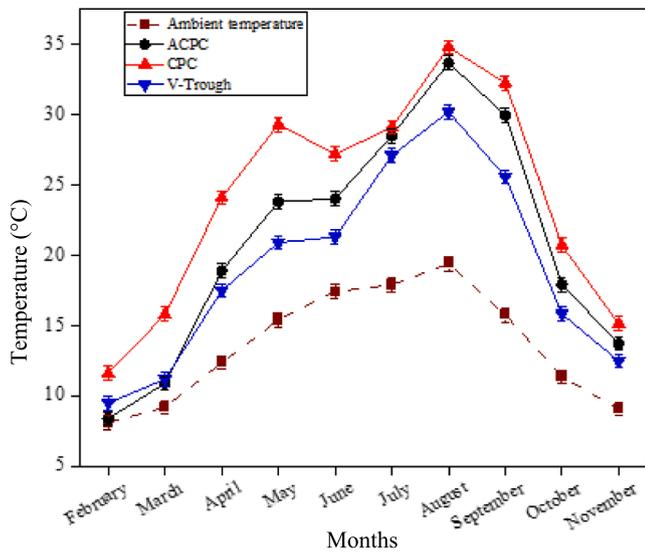
Fig. 8. The monthly average of hourly operating cell temperature of the LCPV panels and the ambient temperature.
