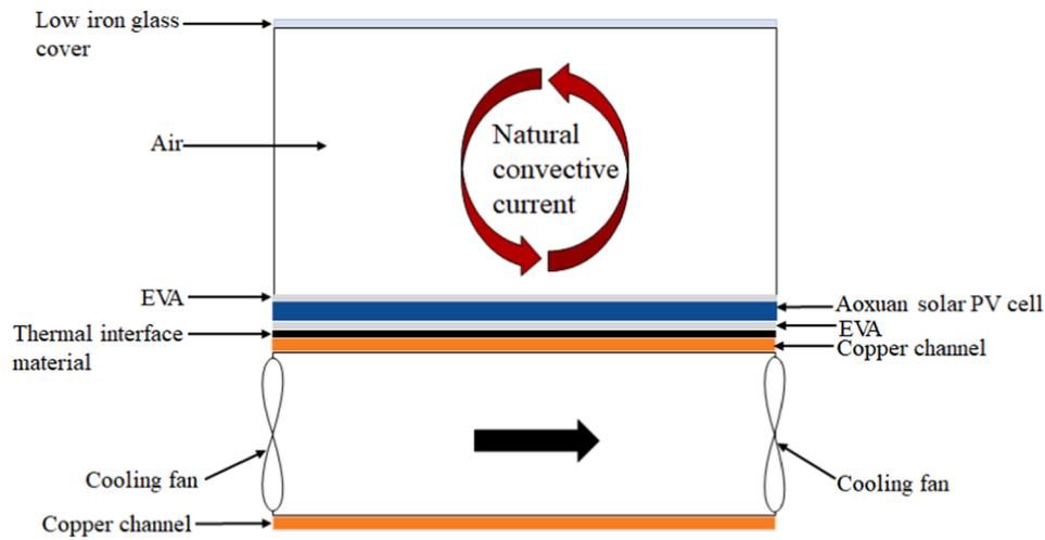
Fig. 2. A cross sectional view of the developed LCPV panel.
