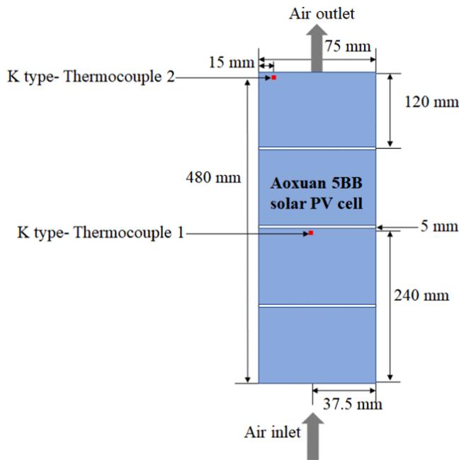
Fig. 3b. Location of the thermocouples under the solar cells.
