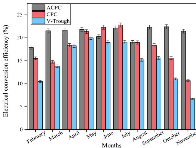
Fig. 12. The electrical conversion efficiencies achieved by the LCPV modules over the monitoring period.
