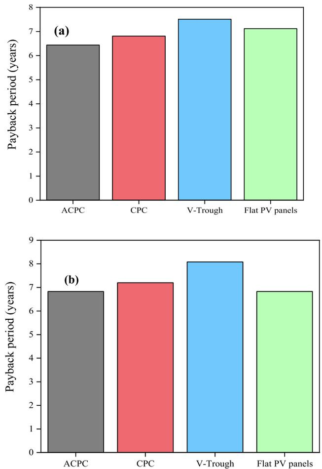
**Fig. 17.** Payback periods predicted for the LCPV and the flat PV panels (a) scenario 1, (b) scenario 2.
