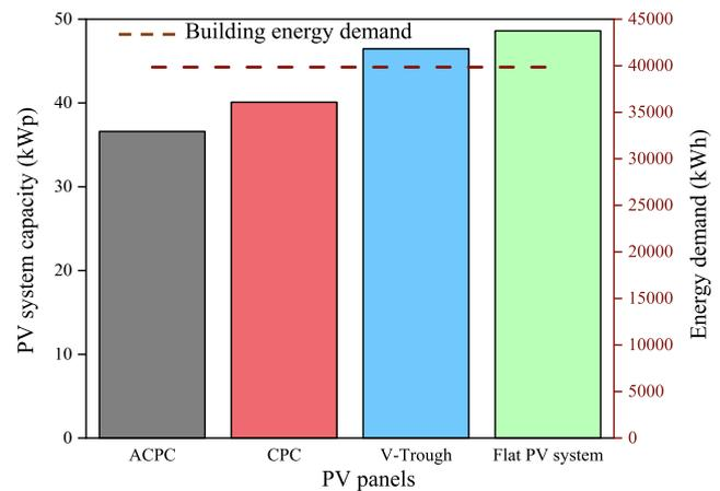
Fig. 16. The comparison of the PV plant installation capacities needed to meet the annual energy demand of the building.
