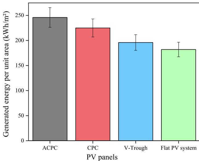
Fig. 14. The generated energy output per unit cell area for the LCPV and flat PV panels.
