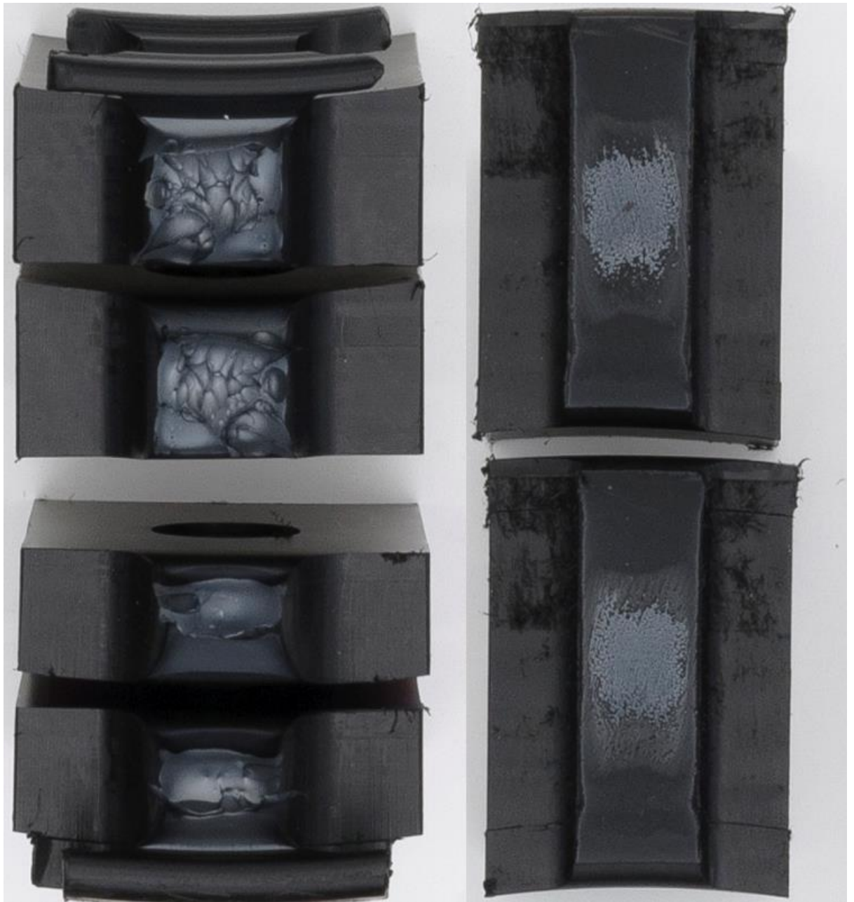
Figure 6-44, Fracture surface for welded modified specimen on the left (PEB233) and welded standard specimen on the right (PEB226) from 630mm OD pipe and from the same weld
