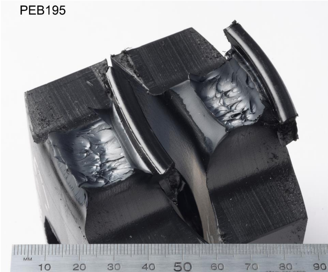
Figure 6-28, Fracture surface of modified welded specimen from 280mm pipe (PEB195)
