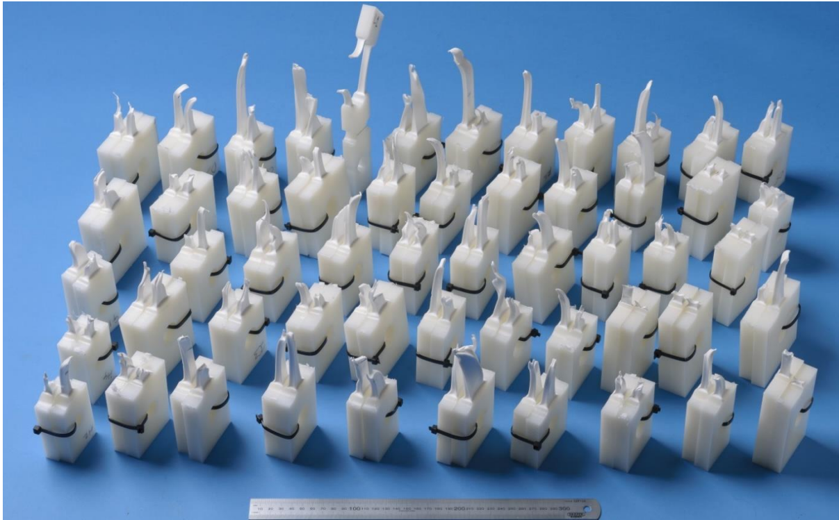
Figure 4-4, Tensile tested specimens for the DOE experiment
