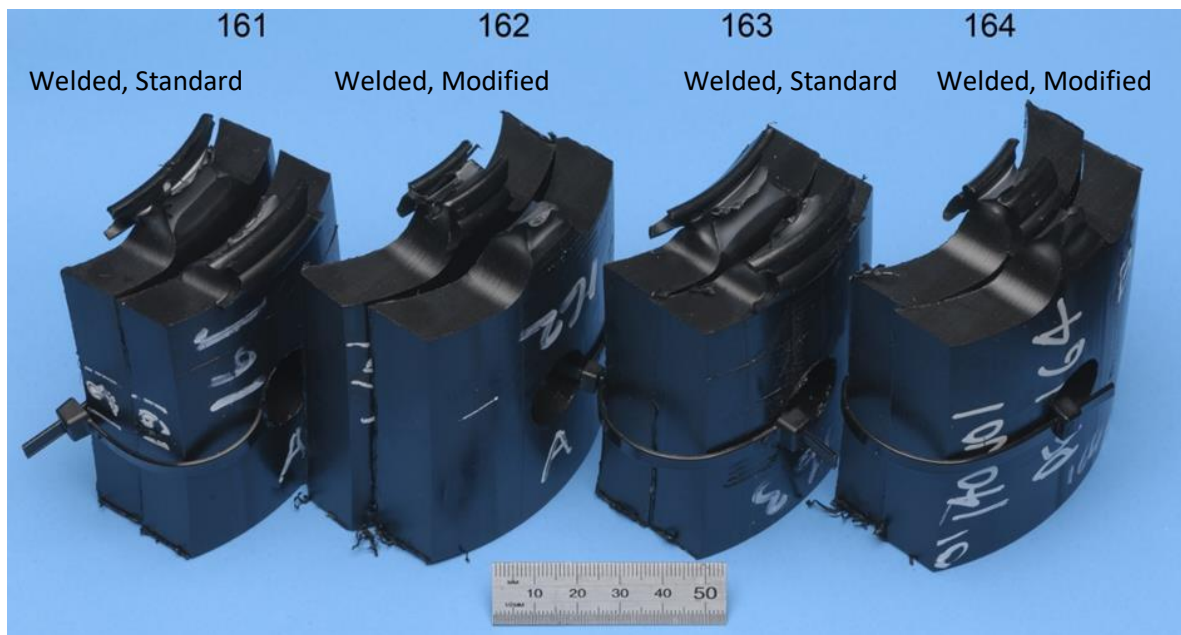
Figure 6-9, From Left, the fracture surface of standard, modified, standard and modified specimen geometry from 140mm OD welded pipe
