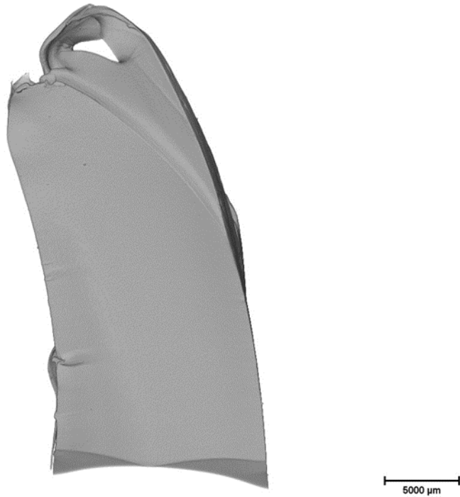
Figure 5-23, X-Ray photography of ductile failure for specimen no 37
