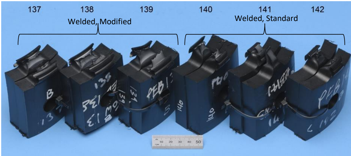
Figure 6-21, From left, fracture surface of modified, modified, modified, standard, standard and standard specimen geometry on 250mm OD welded pipe
