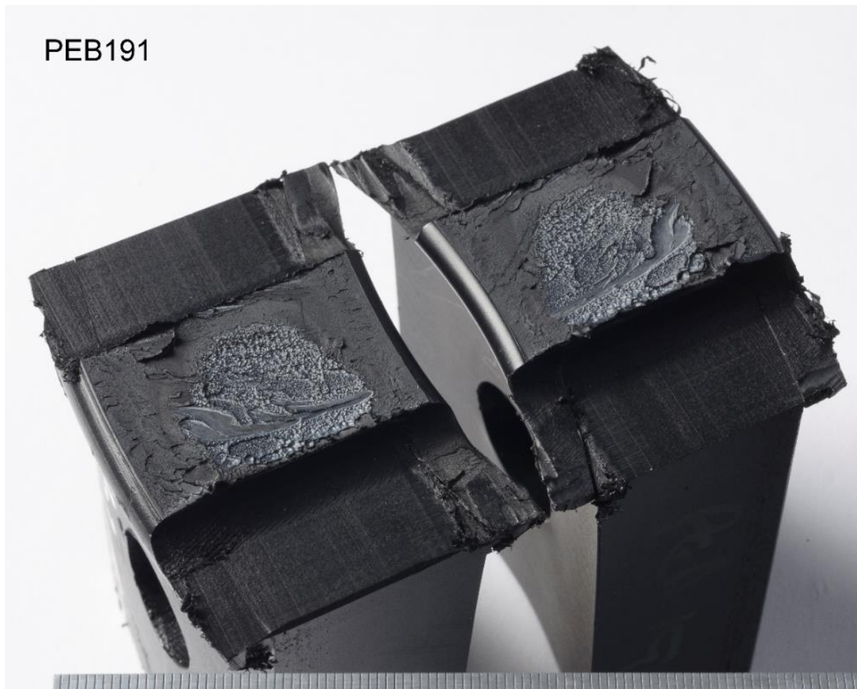
Figure 6-29, Fracture surface of standard welded specimen from 280mm pipe (PEB191)
