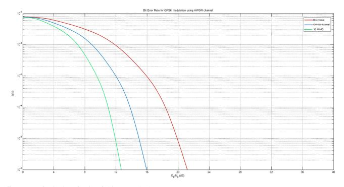
Fig. 14 BER of a signal as a function of Eb/No across the three antenna types
