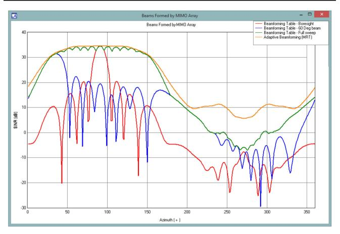
Fig. 11 SINR against Azimuth at various radiation patterns
