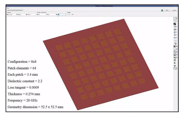
Fig. 4 The antenna geometry and specification
