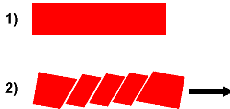
Figure 5-7: Diagram showing 1) an un-loaded, un-deformed specimen and 2) the same specimen after loading has been applied and plastic deformation has occurred. The direction of loading is indicated by the arrow (Anon., 2013).
