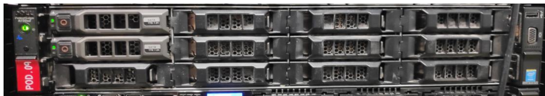
Figure 3-1 Actual picture of the Dell R730xd server
