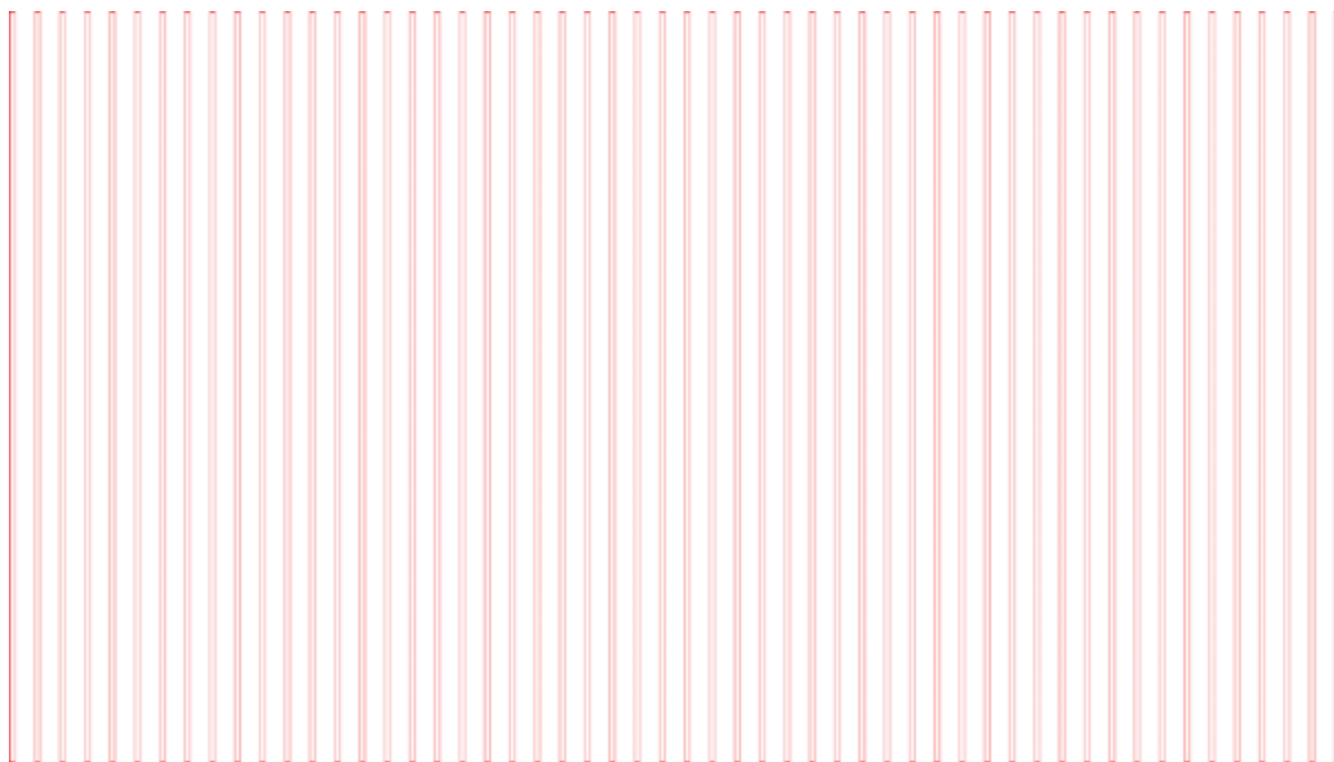
Fig 3.8 - Design of parallax barrier, red rectangle represents the cutting area (Pinhole), white area shows the black area.
