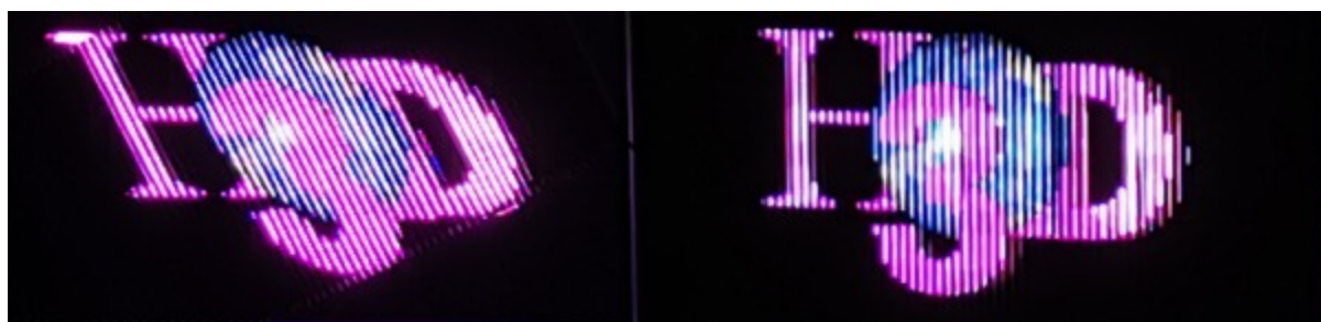
Fig 5.18 - Comparison of playback result of two-pixel mapping methods in the same viewpoint-4, left: Improved 10 views pixel mapping method, right: Classic 5 views pixel mapping method.
