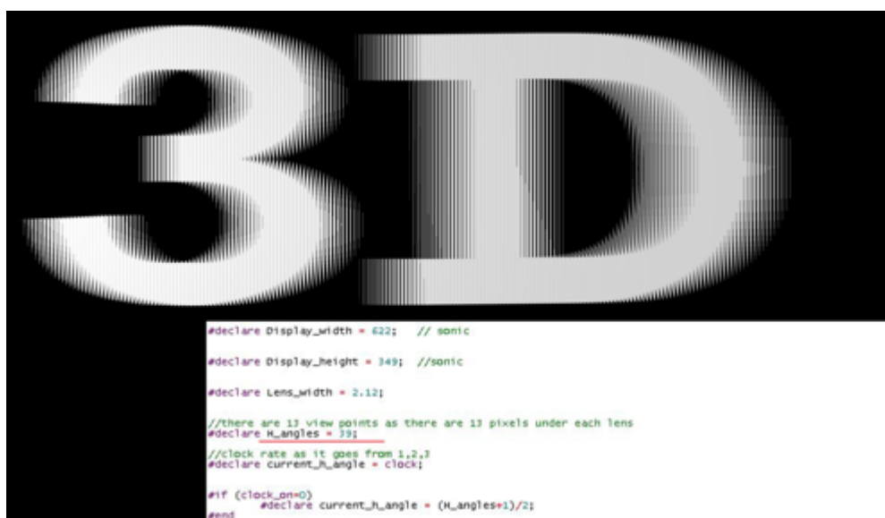
Fig 4.10 - H3D camera's setting with distributed resampling method by changing H_angle from 13 to 39.
