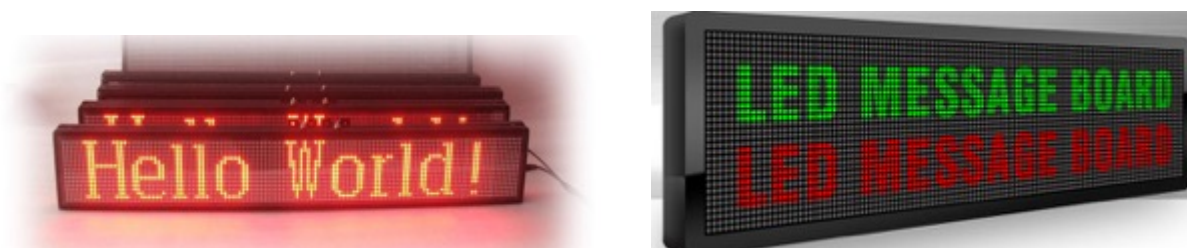
Fig 2.23 - Left: Single colour LED panel (b) Right: Double Colour LED text board.
