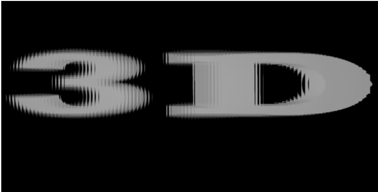
Fig 4.12 - Stitched omnidirectional H3D image which sampling vertical pixel in every three rows, the result shows too less motion parallax in vertical direction.
