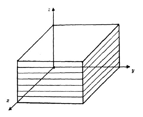
Figure 5.1. An orthotropic material and its (ortho-)coodinate system.
