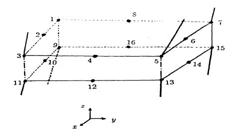
Figure 4.1. A 2D joint element parallel to the x-y plane.
