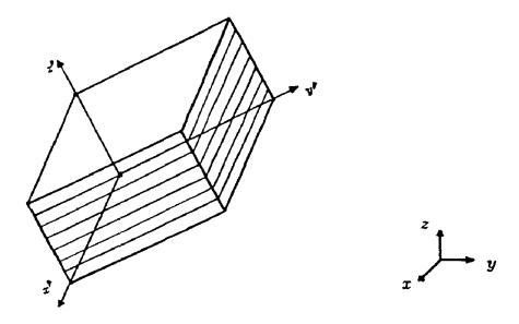
Figure 5.2. An orthotropic material in the *x*-*y*-*z* coodinate system.
