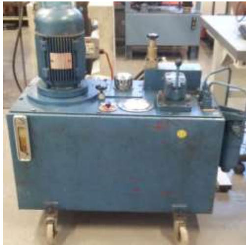
Figure 51: Hydraulic Power Unit
