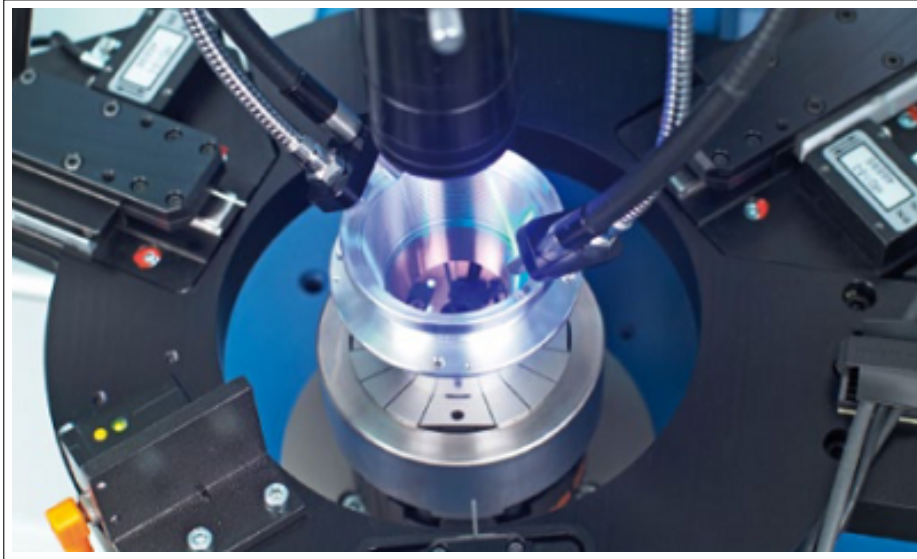
Fig. 2.17 Photography of bonding station with actuator for alignment of the lenses
