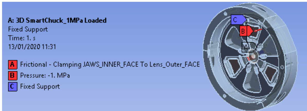
Fig. 4.25 Flexure FL2, FL4 3D FEM setup
