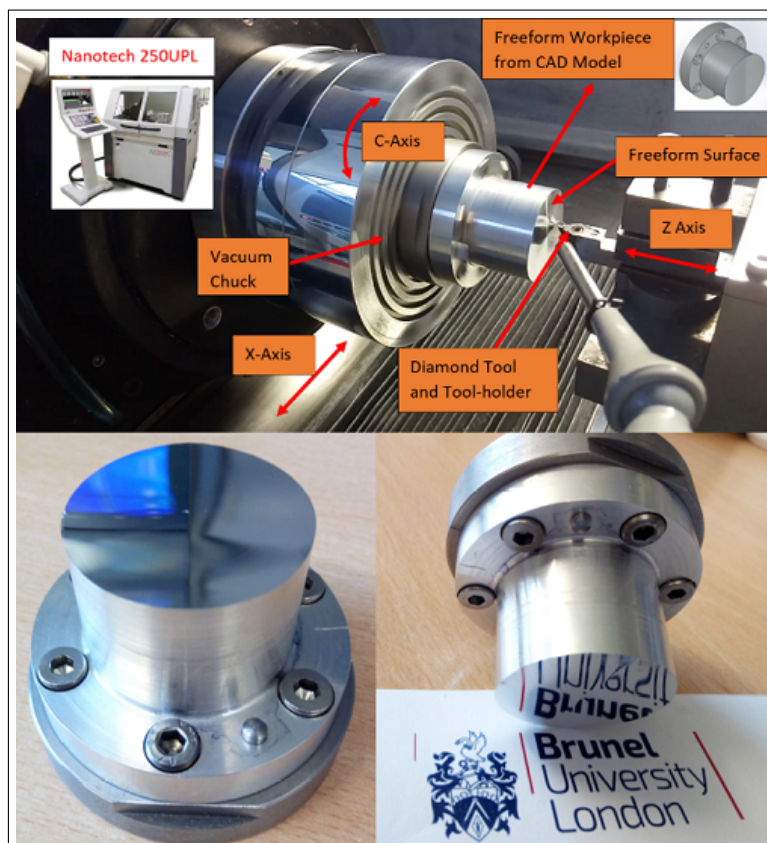
Fig. 3.16 Photograph of the diamond turning machine for the experimental trial and validation of CAM post-processing
