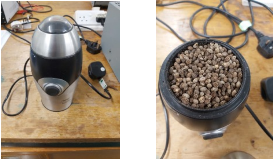
Figure 3. 1: Blender used for milling carica papaya seeds
