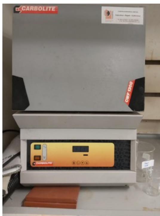
Figure 3. 2: CARBOLITE 1100°C & 1200°C Rapid Heating Laboratory Chamber Furnace used for the calcination of adsorbents
