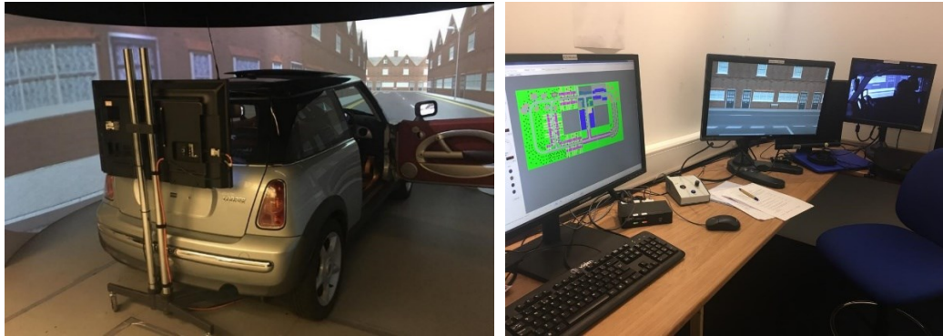
FIGURE 28: BMW MINI BODY SHELL, SCREEN, AND MONITORS AT THE CONTROL ROOM
