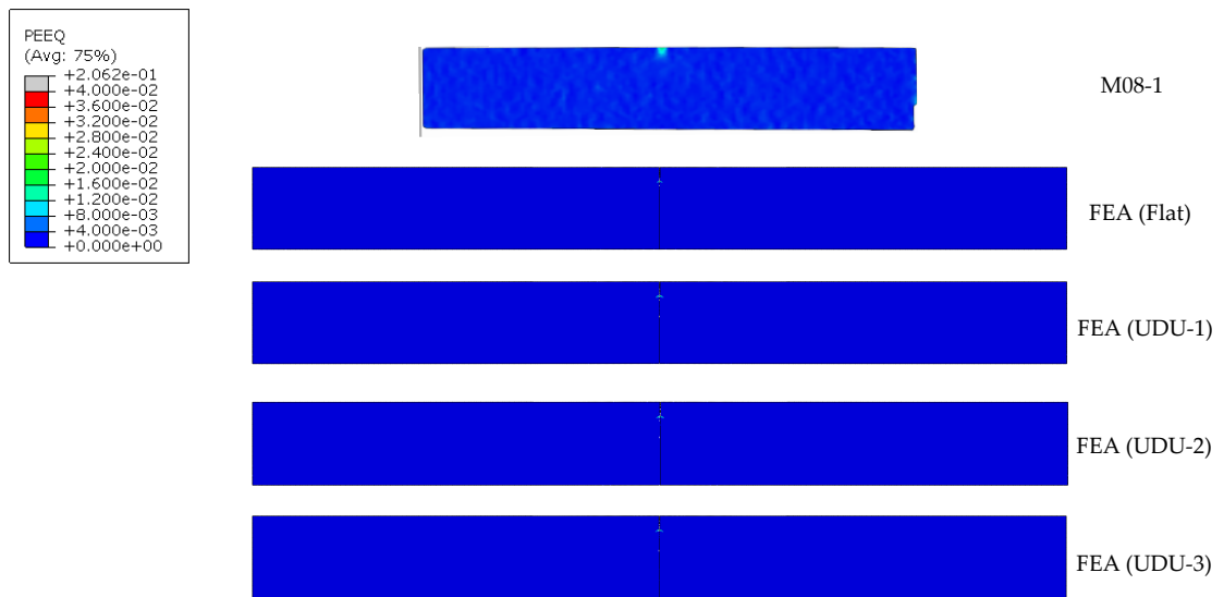
Figure D.7: Comparison between the equivalent plastic strain map calculated from FEA and that from the SENT test (equivalent von Mises strain) at CMOD = 0.031 mm
